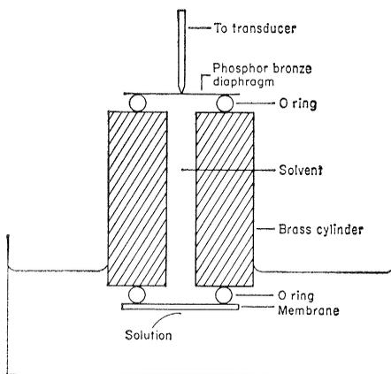
Fig. 3. Hepp-type osmometer. A variant of Hansen's design.
