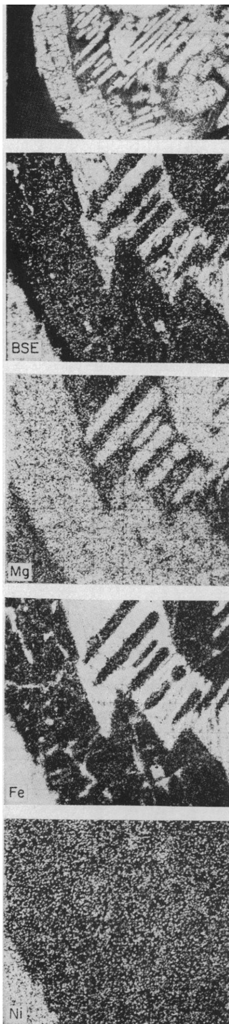
Fig. 6 (left). Photomicrograph and beam scanning pictures of part of a thin section of the Murray carbonaceous chondrite. BSE is a back-scattered electron image and Mg, Fe, and Ni show the distribution of these elements within the scanned area. The chondrule contains alternate lamellae of olivine and a darker, fine-grained, devitrified glass separated from the matrix by a rim of pyroxene. Olivine and pyroxene are both white in the Mg picture, while the devitrified glass with its relatively high iron content shows white in the BSE and Fe pictures. All the chondrule silicates contain much less nickel than the matrix. Scanned area is 250 by 250 \mu .
