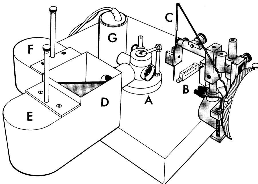
Fig. 1. Layout of the helium-glow photometer. A, Glow chamber; B, sample trough; C, transfer pipette; D, dichroic mirror housing (cover removed for clarity); E, potassium phototube; F, sodium phototube; G, ultraviolet lamp.
