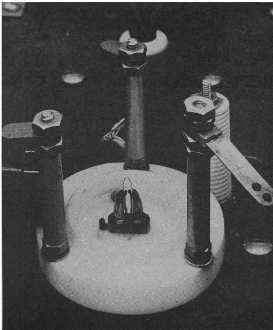
Fig. 2. Details of the lower electrode holder.
