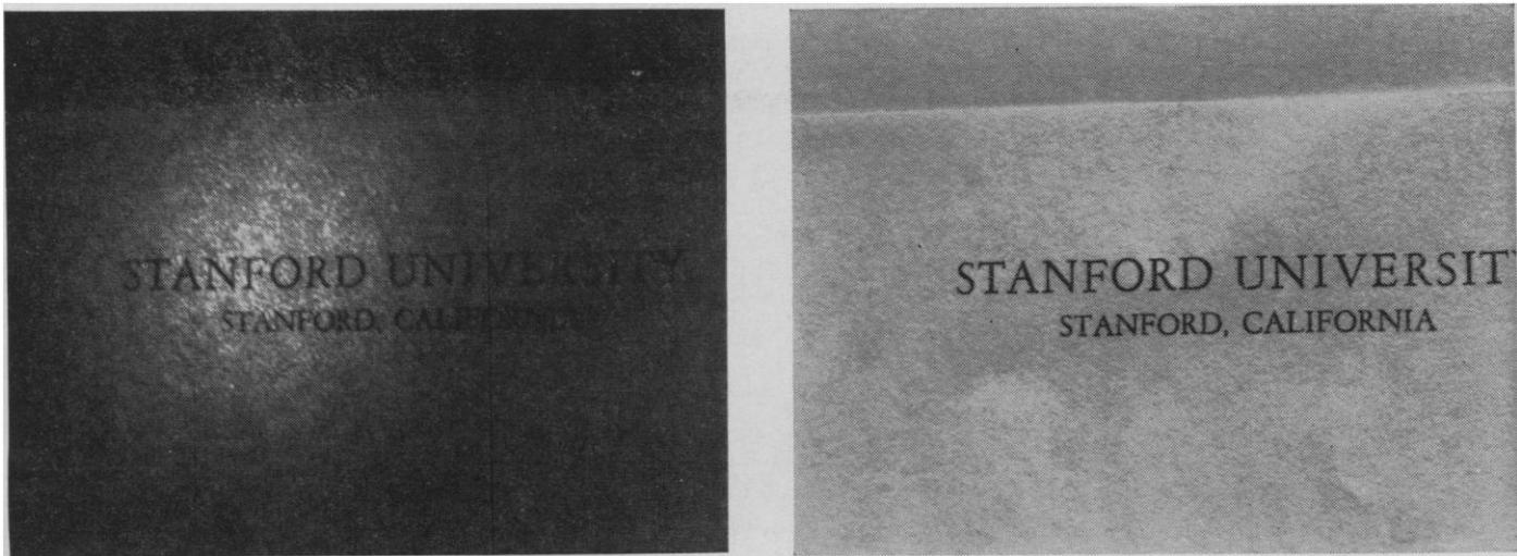
Fig. 2. (Left) A printed piece of paper illuminated by 6328-angstrom coherent light from a gas-discharge laser. (Right) The same paper illuminated by ordinary light.
