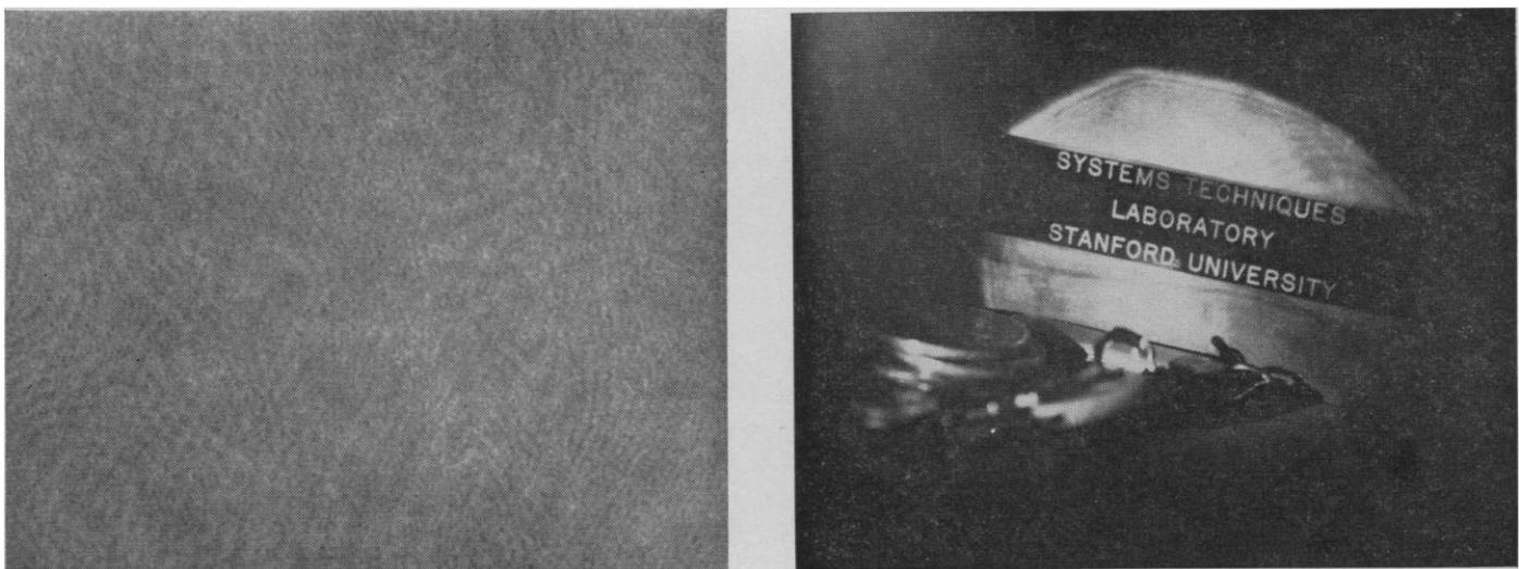
Fig. 3. (Left) A hologram. (Right) The reconstructed image. [Photographs courtesy W. H. Huntley, Jr., D. Jackson, and M. Lehmann]
