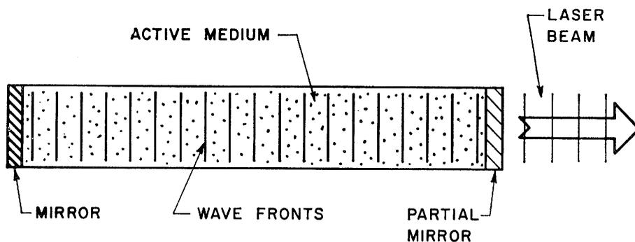
Fig. 1. Basic structure of a simple laser.
