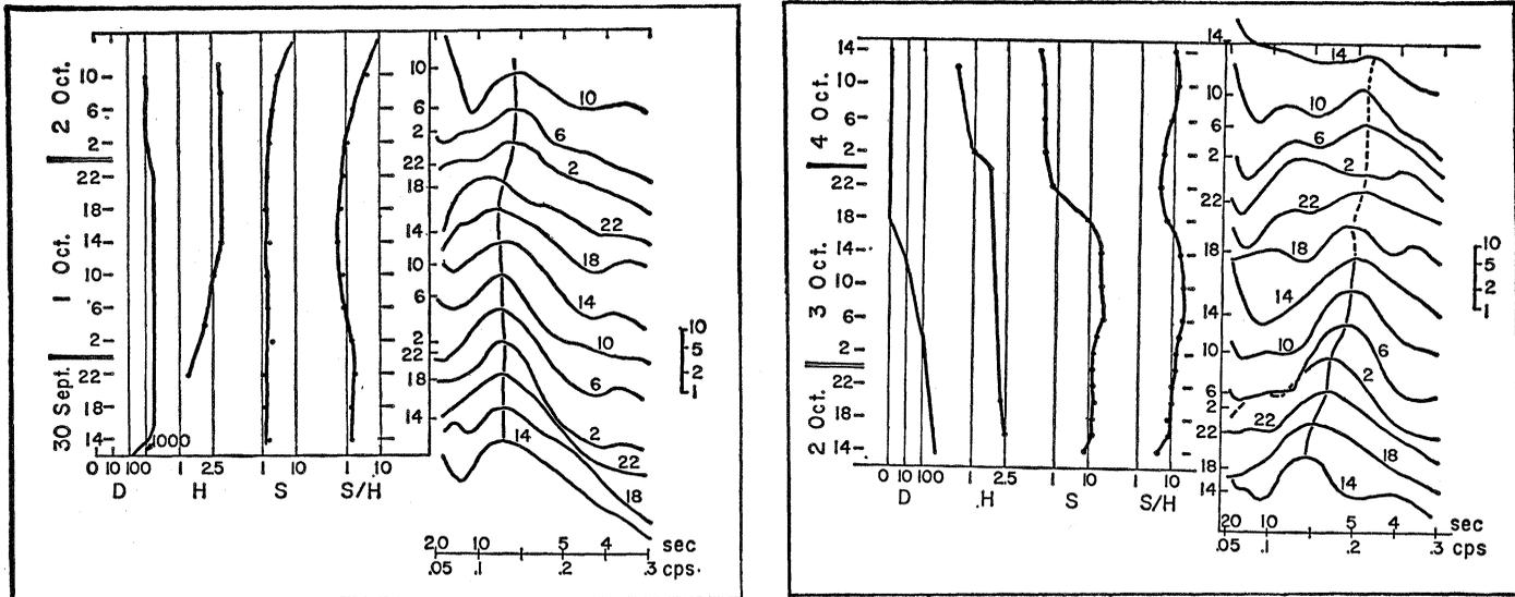
Fig. 2 (left) and Fig. 3 (right). Related measurements along the hurricane track. Times are C.S.T. *D*: water depth in fathoms (1 fathom = 1.83 m); *H*: number proportional to the energy of the hurricane; *S*: number proportional to the seismic energy. The spectra of the microseisms are on the right.
