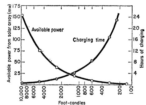
Fig. 1. Graph of power availability and of charging time after 1 hour of use under various light intensities. One foot-candle is equivalent to 11 lumens per square meter.
