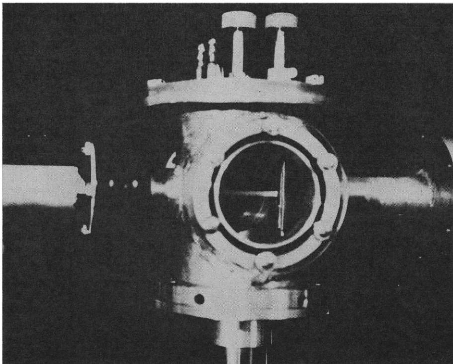
Fig. 7. Photograph of a nitrogen beam, traveling from right to left, being rendered visible by interactions in the carbon foil. There is a high vacuum in the target chamber.
