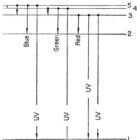
Fig. 1. Some of the energy levels and competing electronic transitions in hydrogen. The length of an arrow is a measure of the energy released as light when the electron moves between the initial and the final states. UV, ultraviolet.
