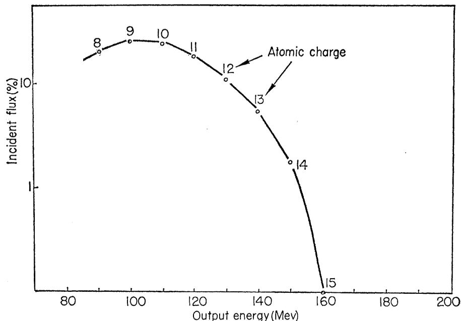
Fig. 3. Ionization distribution resulting from sending singly charged, positive ions of bromine, with an initial energy of  $10^6$  electron volts, through a thin carbon foil. (The abscissa gives the ultimate particle energy following further acceleration of the multiply ionized particles.) [From E. Almquist, M. A. Clark, J. A. Kuehner, A. E. Litherland, *Can. J. Phys.* **40**, 954 (1962)]
