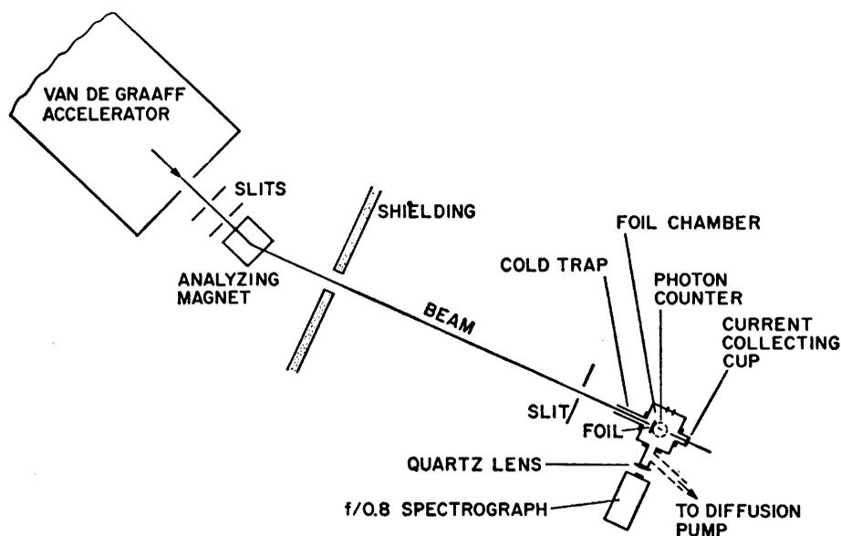
Fig. 5. Schematic diagram of the target arrangement used at the Naval Research Laboratory.
