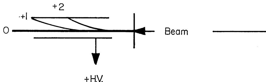
Fig. 9. Schematic representation of beam splitting by electrostatic means.
