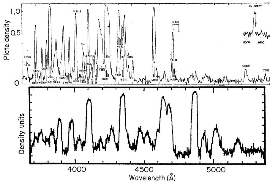
Fig. 4. (Top) Microphotometer tracing of photograph of resolved light from a fast beam of nitrogen and other elements. [From Bashkin and Meinel (4)] (Bottom) Microphotometer tracing of a photograph of resolved light from Nova Herculis 1960. [Data obtained by G. Wallerstein and published by A. B. Meinel, *Astrophys. J.* **137**, 3 (1963)]
