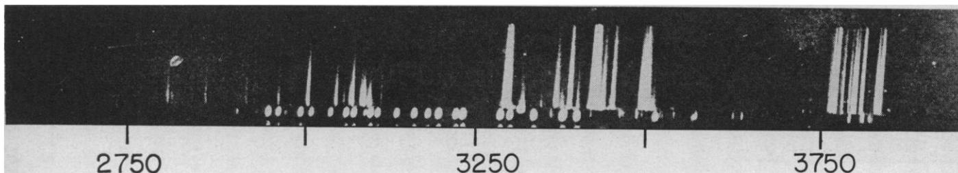
Fig. 8. Spectrum of oxygen, obtained with the beam method. The beam is traveling upward. The carbon foil is at the base of the lines. The blobs below the foil are poorly focused comparison spectra. Wavelengths are in angstroms.
