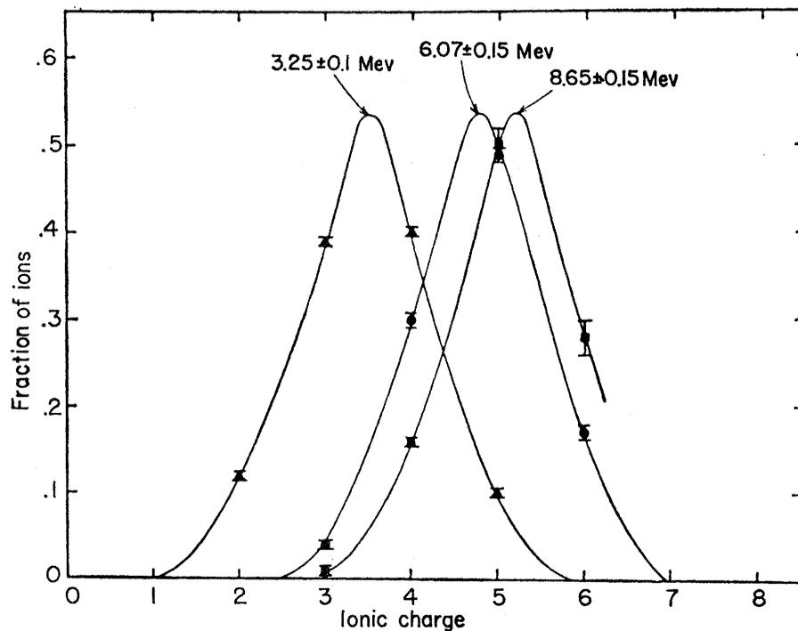
Fig. 2. Ionization distribution resulting from sending singly charged, positive ions of oxygen through argon gas. The three curves pertain to three different incident energies (in millions of electron volts). [From E. L. Hubbard and E. J. Lauer, *Phys. Rev.* **98**, 1814 (1955)]
