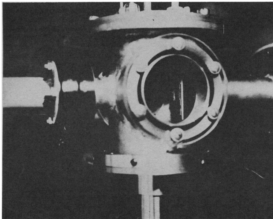
Fig. 6. The target chamber. A lucite window provides a view of the foil holder inside the chamber. The beam enters from the right.
