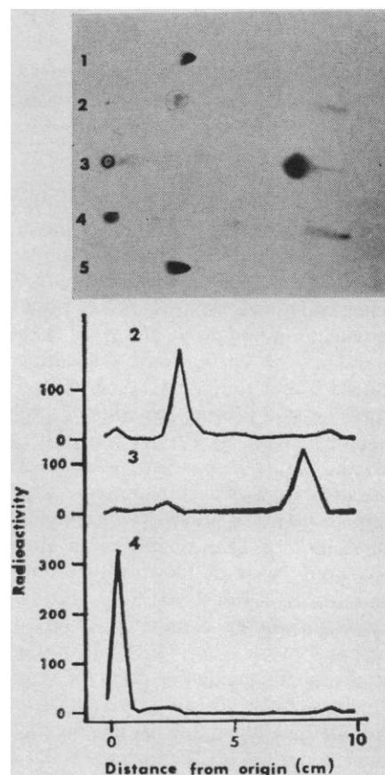
Fig. 1. Chromatographic behavior and radioactivity (count/min) in derivatives of purified fraction III in benzene-chloroform-methanol (4 : 1 : 1). Sample 4 is the untreated metabolite; sample 2, the methyl ester of the metabolite; and sample 3, the silyl ether of the esterified metabolite. Samples 1 and 5 are standards of free retinoic acid.
