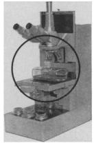
Accepts Specimens to 90mm High The microscope body can be raised on its slide to give a clearance which will accommodate very large objects such as tissue culture flasks and other special experimental set-ups.
