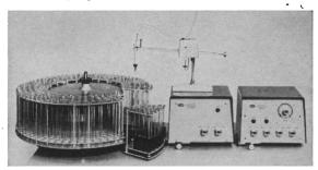
Universal Model, for volumetric siphoning and timedflow collecting in spiral or "square-wave" patterns. Includes Rotator, Distributor, Controller, Siphon Stand, Rimless Tube Racks and Tubing Holder.
