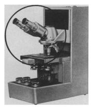
Variety of Beamsplitter/Body Combinations Two beam-splitter boxes are offered one varying instantaneously from 50% visual 50% camera to 100% camera the other 100% visual to 100% camera. Monocular or binocular bodies fit as required to prism box in use.
