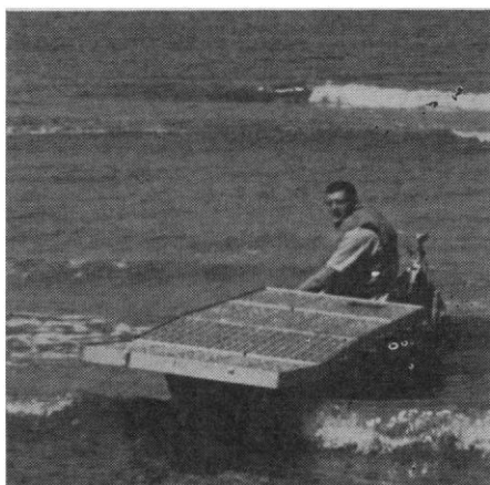
Boat with solar cell panels mounted on deck (left) negotiates light surf at Fort Story, Va. Solar boat developer John Hoke is aboard. With one panel mounted overhead (right), boat is tested on tidal river with one motor operating during Army tests.
