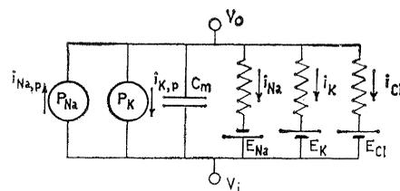
Fig. 1. Equivalent electric circuit of the membrane.  $E_{Na}$ ,  $E_K$ , and  $E_{Cl}$  are the equilibrium potentials of  $Na^+$ ,  $K^+$ , and  $Cl^-$ , respectively;  $C_m$  is membrane capacity;  $i_{Na}$ ,  $i_K$ , and  $i_{Cl}$  are the passive currents of  $Na^+$ ,  $K^+$ , and  $Cl^-$ .  $P_{Na}$  and  $P_K$  are ion permeabilities;  $i_{Na,p}$  and  $i_{K,p}$  are the currents generated by the Na and K pumps;  $V_o$  and  $V_i$  are potentials outside and inside the membrane.
