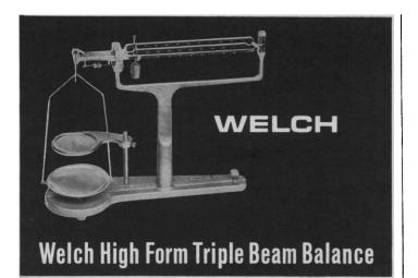
Highly sensitive . . . to 0.01 gram. Capacity is 111 grams and can be increased to 201 gr. with the extra weight. Adjustable platform for specific gravity determinations.
