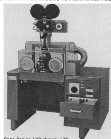
Sage Series 100 shown with Zeiss WL microscope; Incubator and large capacity film magazine are optional accessories
