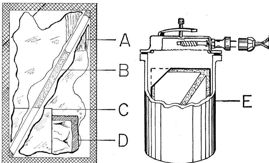
Fig. 1. (Left) A cutout view of the hydrogen generator. A, Coarse filter; B, heat seal; C, fine filter; D, absorbent paper bag containing chemicals. (Right) E, Position taken by generator in the anaerobe jar.
