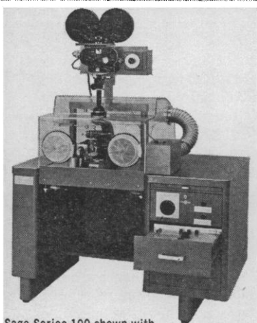
Sage Series 100 shown with Zeiss WL microscope; Incubator and large capacity film magazine are optional accessories
