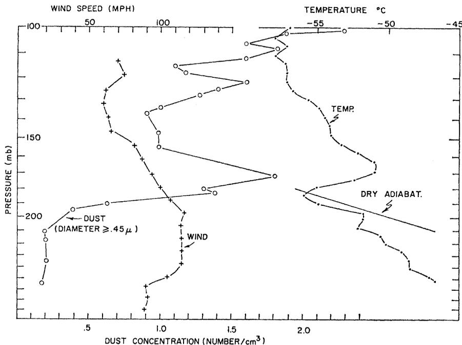
Fig. 3. Fine structure of the dust, wind, and air temperature obtained between 300 and 100 mb on flight 719, 18 August 1964.
