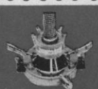
HHS Vacuum Heating Stage for 1500° C. $625
