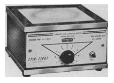
Equally good as a light box or a magnetic stirrer, Stir-Light combines the best features of both uses to promote accurate and speedy titrations, slide work or visual inspections.
