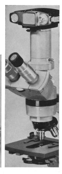
It's no longer necessary to accept photomicrographs that are crisply in focus only in a small, pre-selected area of the field of view. The new AO Microstar® Microscope's unique infinity-corrected optics provide a visual image that's amazingly flat over the entire field. This superior image quality means you now can make photomicrographs that are flat and in focus from edge-to-edge and corner-to-corner of the print.
