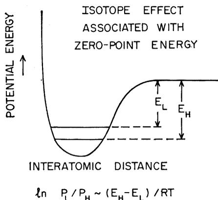
Fig. 1. Schematic potential-energy curve for the interaction of two atoms in a stable molecule or between two molecules in a liquid or solid.
