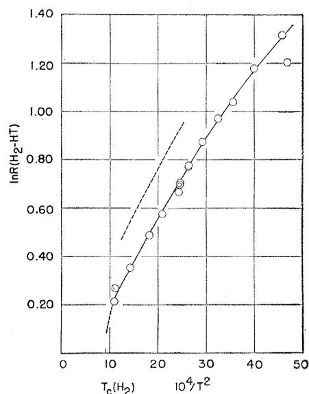
Fig. 5. Distribution coefficient for HT, in solution in  $H_2$ , between liquid and vapor as a function of temperature. Dotted curve is that calculated for a solution of  $D_2$  in  $H_2$ . [From Bigeleisen and Kerr (8), courtesy *J. Chem. Phys.*]
