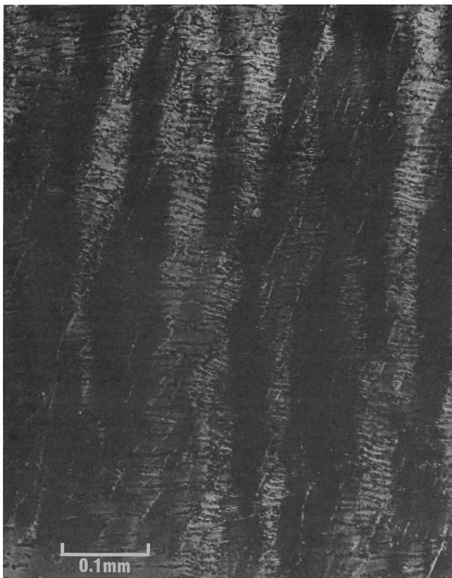
Fig. 3 (top left). Specimen DT-140 photographed in phase contrast illumination between crossed nicols. N-S bands are remnant kink bands subparallel to the c -axis. E-W worm-like features are recrystallized basal lamellae. The less prominent NNE trending features are recrystallized lamellae whose traces on the section are inclined 5° to 25° to the c -axis. At low temperature, specimen formed prismatic kink bands by basal slip. As the temperature was raised, stress relaxation was accompanied by recrystallization.
