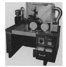
Sage Series 100 shown with Zeiss Plankton microscope. Includes built-in Xenon light source for high intensity flash photography. Incubator optional. from \$6750
