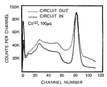
Cs<sup>137</sup> spectra accumulated at high counting rates with and without pileup rejection circuit.
