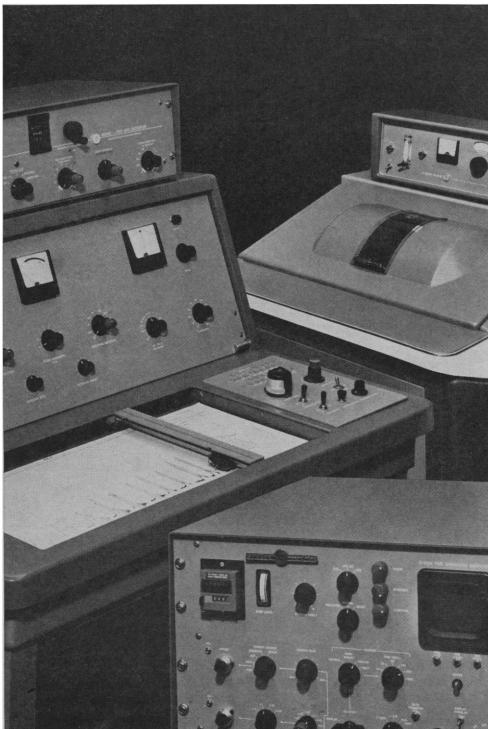
That first A-60 spectrum of a 0.10% ethyl benzene solution is so noisy that it is almost worthless. So we reran the sample a hundred times, using an A-60 spectrometer equipped with our new C-1024 time averaging computer. The second spectrum shows the result: a clear, readable, useful signal which has improved the signal-to-noise ratio by a factor of 10.
