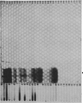
Purified protein components can be recovered from high-resolution gel-electrophoresis patterns by elution-convection electrophoresis. The protein components are all simultaneously eluted from the gel pattern and are simultaneously concentrated to recover the proteins in the original undiluted concentration.
