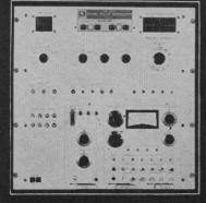
The new RIDL Nanolyzer\* offers two principal advantages over other presently available multichannel analyzers: speed and accuracy. It can accept, analyze, and store data seven to fifty times faster than conventional analyzers. It will also store at rates of over 200,000 counts per second with a minimum of distortion when Nal(TI) detectors are used. These benefits are obtained by using several totally new circuit concepts, chief among which are those described at the right.
