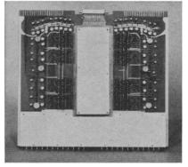
Plug-in circuit board with 128-word thin-film memory plane.
