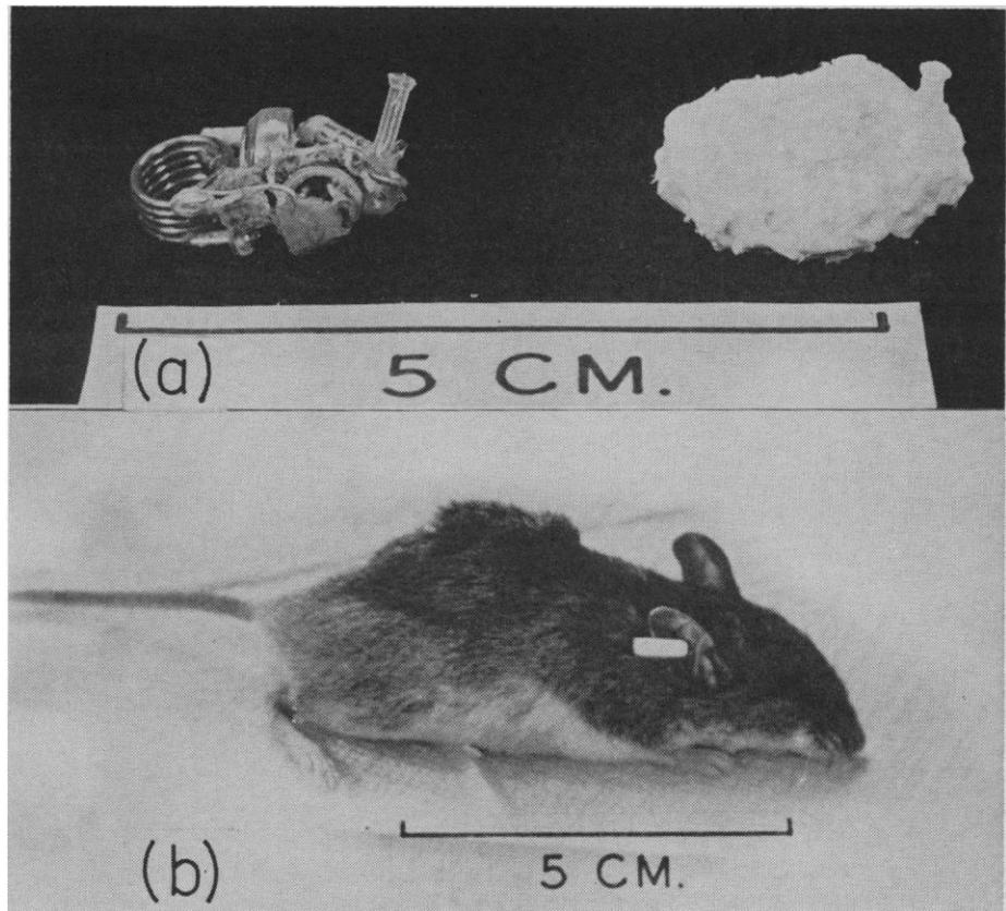
Fig. 2. Radio transmitter for mice. (a) Before and after encapsulation in white silicone rubber. (b) After implantation in a mouse, showing the deformation of the dorsal contour. The photograph is of an anesthetized animal immediately after the operation; the mouse carries a numbered metal ear tag.
