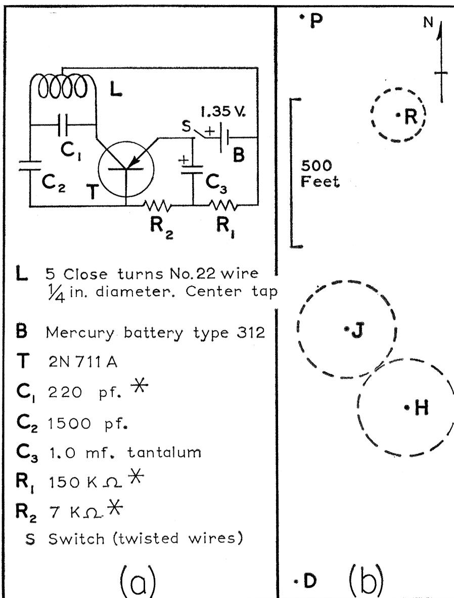
Fig. 1. (a) Schematic circuit of the transmitter. Ferrite chips are placed within the coil  $L$  for final radio-frequency tuning. Values marked \* are typical and must be adjusted for each circuit (pf, picofarad; mf, microfarad; k $\Omega$ ,  $10^3$  ohms). (b) Map relating release points to home (H) for the homing experiments described. Dashed circles show the approximate ranges of the receiver antennas (500 feet is equivalent to 152 meters).
