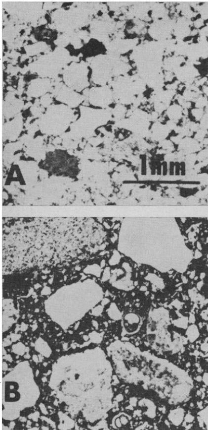
Fig. 1. Photograph of a thin section through (A) core V 7-42 (135 cm), subarkose-type sand; and (B) core V 7-55 (355 cm), graywacke-type sand ( $\times 25$ ). Light-colored grains are quartz and feldspar. Note abundant dark-colored interstitial matrix in B. The thin sections are obtained from portions of cores that have been impregnated with epoxy resins, sliced, mounted on glass, and ground to the standard thickness of  $30 \mu$ .
