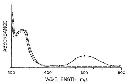
Fig. 1. Ultraviolet and visible absorption spectra of 2-(2,4-dinitrobenzyl)pyridine in PVA: spectrum at  $-185^{\circ}\text{C}$  before irradiation, —; spectrum at  $-185^{\circ}\text{C}$  after irradiation for 120 seconds at  $-185^{\circ}\text{C}$ , ---; spectrum of colored form at  $-91^{\circ}\text{C}$  after irradiation for 120 seconds at  $-185^{\circ}\text{C}$ , -.-.
