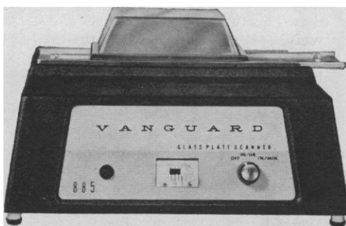
Designed as an accessory to operate with Model 880-D, the Model 885 Glass Plate Scanner provides a convenient, low cost system to assay TLC glass plates with unequal accuracy and sensitivity.
