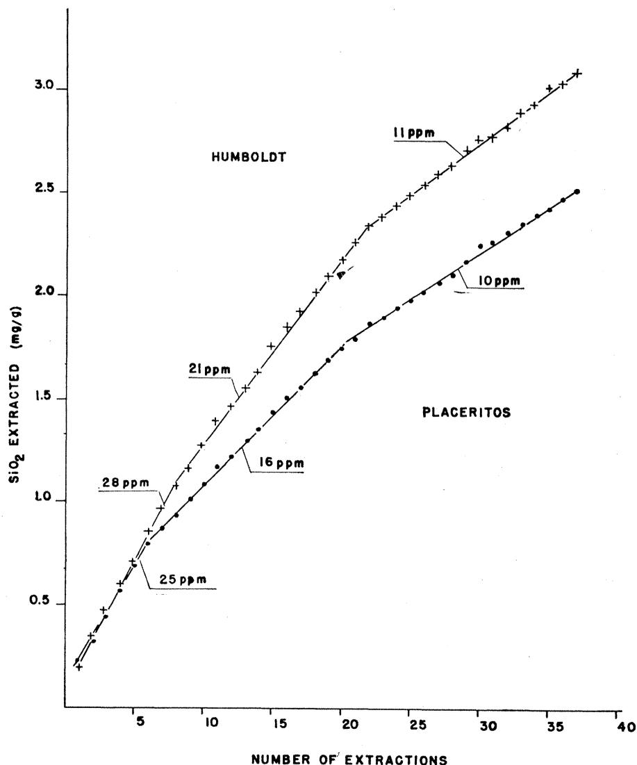
Fig. 1. Relation of number of 130-ml extractions to total  $\text{SiO}_2$  extracted from 30-gram samples of two soils. The concentrations shown are the mean concentrations of the extracting solution calculated from the slopes of the straight lines.
