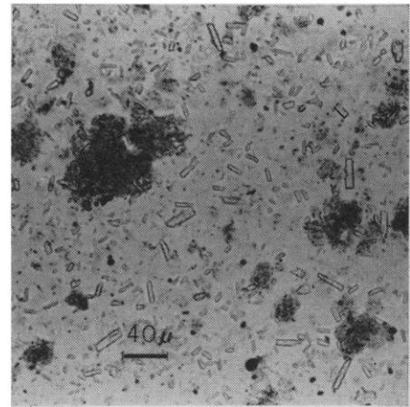
Fig. 1. Photomicrograph of zeolite crystals.
