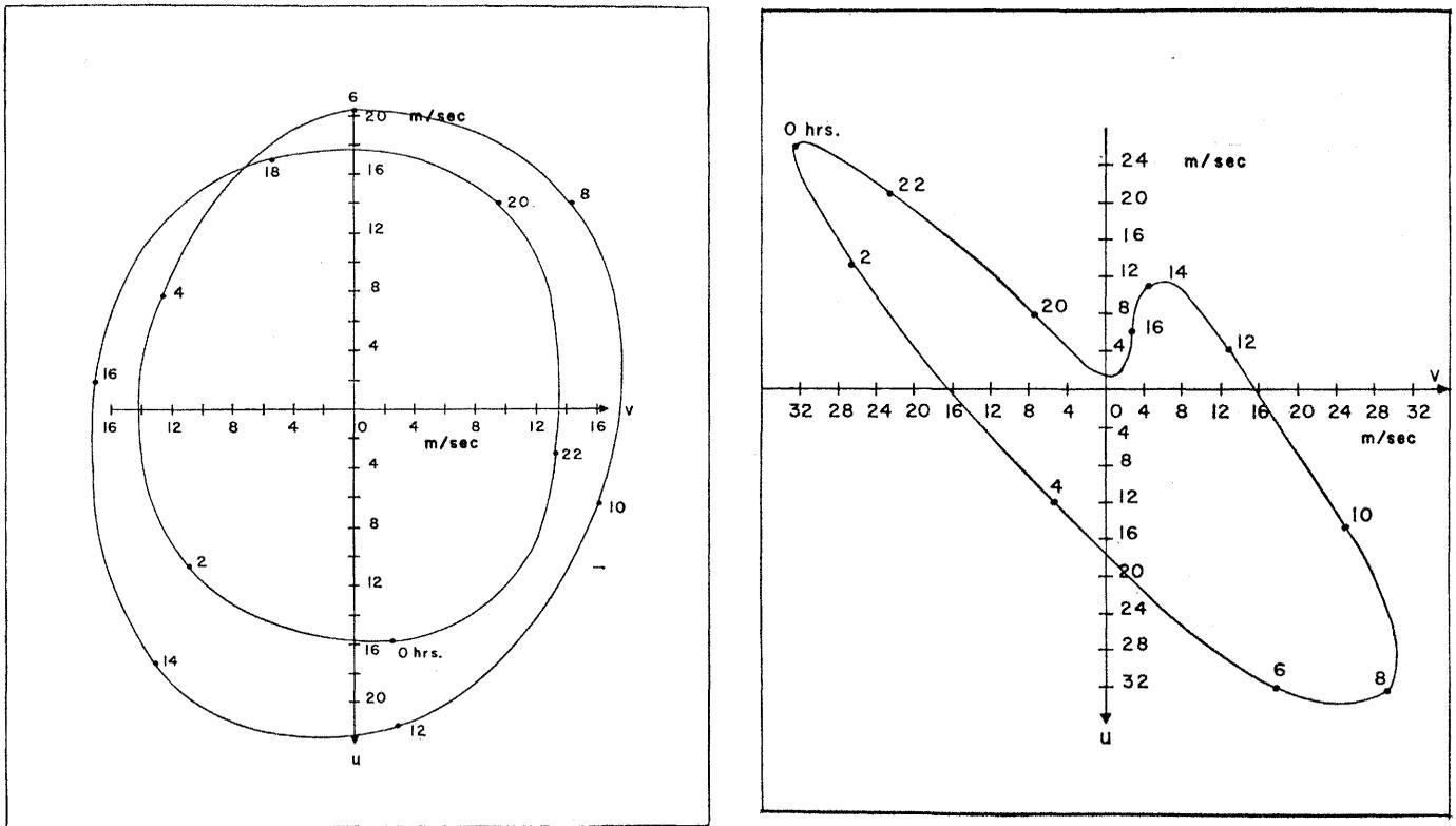
Fig. 6. Hodographs of the periodic components ( $S_1 + S_2$ ) of the wind vector at altitudes of 80 to 100 kilometers during the  $D$  months (November through February), in meters per second, at (left) Jodrell Bank, England and (right) Adelaide, Australia. The curves represent the end points of the periodic wind vectors. The numbers adjoining the curves are hours, in local mean time.
