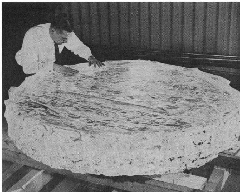
Fig. 5. The rough silica blank for the primary mirror being examined at the Bradford plant of Corning Glass Works shortly after it was taken out of the furnace. [Corning Glass Works]
