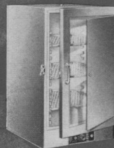
Cat. No. 400 INCUBATOR. Range to 65°C. Interior 18" W x 27" H x 18" D. 3 shelves, hot wall heat. . . . $265.00
