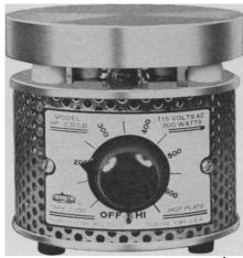
Precise, stepless thermostatic control, from 6°C above ambient to 370°C (700°F)
