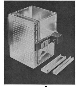
Using Cyanogum, preparation is simplified—completed patterns are transparent, flexible, and easily stored. Pore size can be regulated . . . electrosmosis eliminated.
