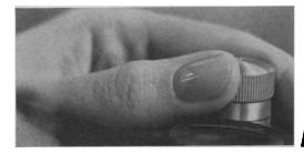
achieving a desired magnification using a lower power objective and the plus magnification of the DynaZoom system you increase the working distance—the real field-of-view is increased—the depth-of-focus is increased and you have a much flatter field of view.
