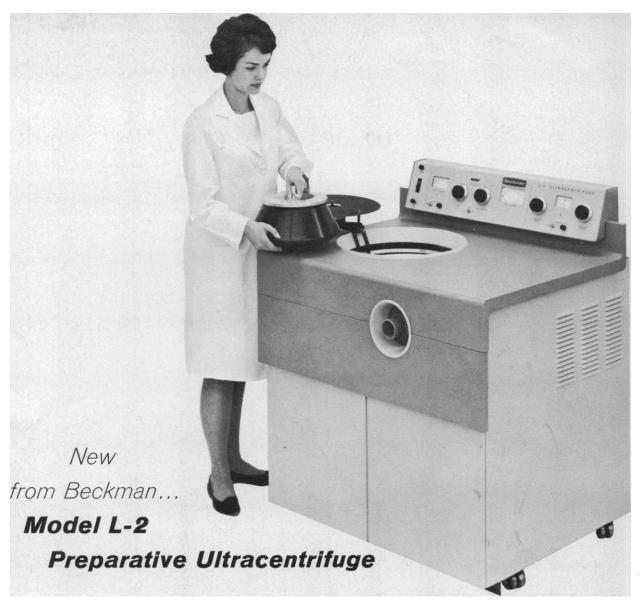
Here is an advanced instrument for preparative centrifugation. More sophisticated than our Model L, the new L-2 has a substantially larger rotor chamber which holds not only every Model L rotor, but bigger swinging-bucket and fixed-angle rotors with far larger sample volumes. It has a convenient system to control rotor temperature, and it has a stabilizer to prevent rotor wobble during deceleration, helping to keep fractions from remixing.
