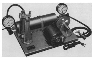
For catalytic reduction, condensation and other reactions with hydrogen
