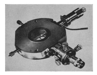
Two-dimensional lateral displacement and two independent angular movements of the specimen under investigation are possible by replacing the standard specimen stage with the rotating/tilting specimen stage.
