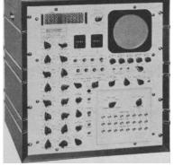
● Model ST-400DM\* 400-Channel Analyzer 106 or 105—1 counts/channel Up to 4 inputs with differential data accumulation
