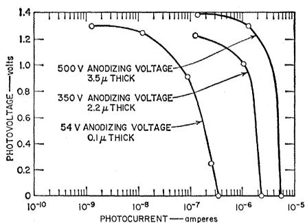
Fig. 1. X-ray induced bulk photovoltaic effect in cells of  $Ta_2O_5$  with Ta and Au electrodes.
