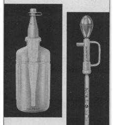
The Nalgene Safety Pipet Filler takes the hazard out of handling volatile, corrosive, poisonous liquids —eliminates the danger of mouth contact. Draws up any quantity . . . dispenses precise amount. Unbreakable, corrosion proof, chemically inert. Compact and lightweight—easily operated with one hand. Fits snugly over top of pipets up to 20 ml sizes. Price, each . . . . . . . . . \$4.50 Be safe . . . be sure . . be accurate with Nalgene Pipetting Aids.
