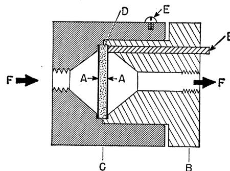
Fig. 1. Cross section of the hygrometer. A, Porous stainless steel capacitor plates; diameter, 1.5 cm; spacing, 2.0 mm. B, Teflon plug. C, Stainless steel body. D, Packing material. E, Electrical connections. F, Airflow.
