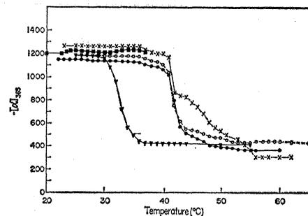
Fig. 1. Denaturation of collagen in solution measured by optical rotation. Solid triangles, acetate ionic strength, 0.15; pH 4.2. All other curves represent collagen in phosphate ionic strength, 0.4; pH 7.6 with varying concentrations of arginine. Closed circles, 0.4M arginine; open circles, 0.2M arginine; X-X, 0.1M arginine; solid squares, no arginine.
