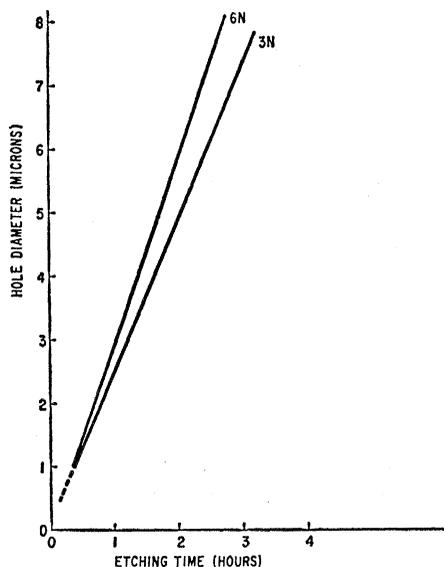
Fig. 2. Etching characteristics of polycarbonate film in unstirred aqueous solutions of 6N and 3N NaOH at 75°C. The film thickness decreases as the hole size increases, so that a film containing 6- $\mu$  holes has been reduced in thickness by about 6  $\mu$ .
