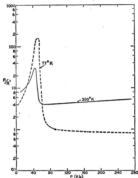
Fig. 1. Resistance of ytterbium as a function of pressure, at 77°K, and as a function of pressure and change of temperature to 300°K. Resistances are values of the ratio  $R/R'$ , where, for both curves,  $R'$  = resistance at 77°K and 100 kb.
