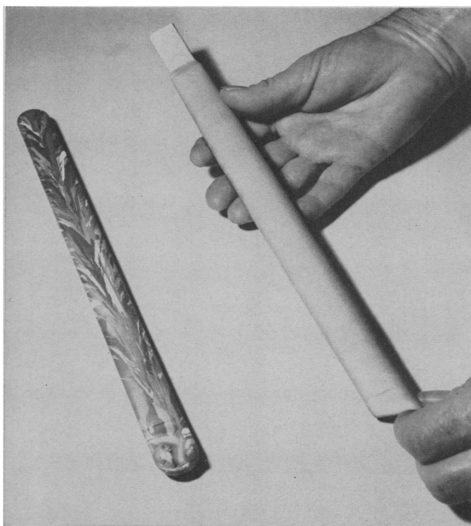
Fig. 6. At left, polycrystalline zone-refined germanium ingot; at right, zone-leveled single crystal germanium ingot. [Bell Labs. Record (June 1955)]
