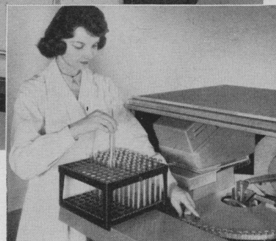
A sliding cover over loading compartment makes a convenient counter for handling racks of test tubes.
