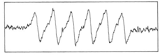
Electron paramagnetic resonance in aqueous solutions is complicated by the fact that water has a high dielectric loss at typical microwave frequencies. The V 4501 Spectrometer employs a rectangular TE<sub>102</sub> resonant sample cavity. The difficulty of dielectric loss in this sample cavity can be overcome by using a flat sample cell which constrains the sample in the nodal plane of minimum r-f electric field (and maximum r-f magnetic field).
