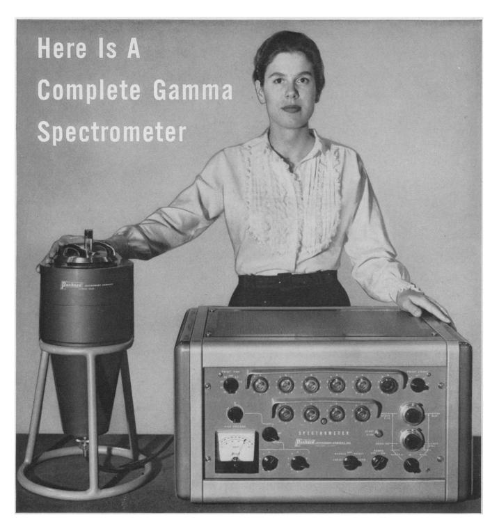
This transistorized spectrometer is by far the smallest and most compact available—yet it has more important and unique features than any other on the market today. Furthermore, it can be used directly with the Packard Auto-Gamma Sample Changer for completely automatic counting of test tube samples.
