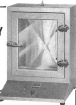
Model CD-4 is a thermostatically controlled, insulated oven which quickly reaches temperatures up to 110° C. Achieves evacuation of solvent vapors with water or motor aspirator. Heating elements concealed in base are protected from combustible, solvent droplets. Heavy metal-reinforced safety glass door readily permits temperature readings and observation without repeated opening of door. Stainless steel oven chamber is corrosion-resistant.
