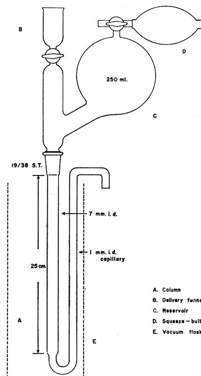
Fig. 1. Assembly for low-temperature chromatography.
