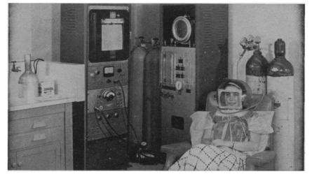
**DETECTS AS LITTLE AS 10<sup>-12</sup> CURIES**—The high sensitivity and high precision of the Cary Model 31 Electrometer permit minimum amounts of costly "tagged" materials to be used in radioactive isotope studies, saving enough to pay for the instrument in a short time and materially reducing the hazard to living experimental subjects.
