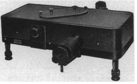
with exchangeable prisms for the visible, ultraviolet, infrared from 200 millimicrons to 20 microns
