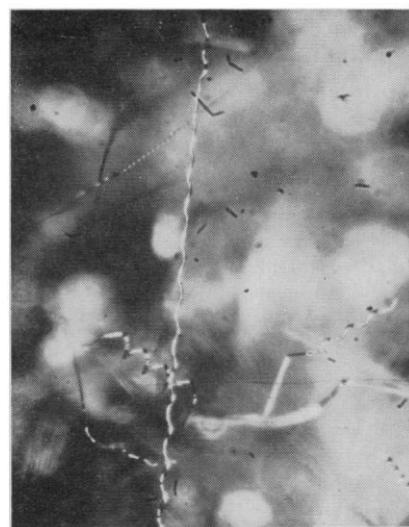
Fig. 2. Portion of a cluster of palladium whiskers. Note the helices of slowly varying pitch and the abrupt transitions of pitch. Several helices are composed of connected straight segments. The length shown of the long helix is 0.8 mm.
