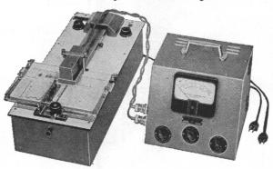
A photoelectric precision instrument for the rapid and convenient evaluation of strips and sheets of filter paper in partition chromatography and paper electrophoresis.
