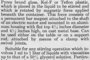
volves 1 ml to 1 liter of liquids with viscosities up to that of a 50% glycerol solution. Particularly convenient for use in closed systems. Any type of vessel of glass, porcelain or nonmagnetic metal can be used.
