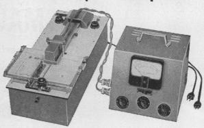
A photoelectric precision instrument for the rapid and convenient evaluation of strips and sheets of filter paper in partition chromatography and paper electrophoresis.
